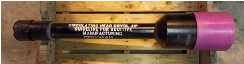
Figure 11: Picture of a circulating head produced by WAAM during the development of the DNV-GL guideline [2] . Manufacturing and tests were led by Vallourec. Length about 1.2 meters.
